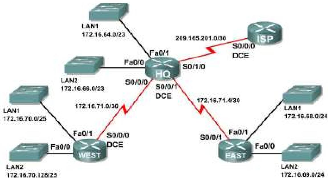
Determine summarized routes that can be used to reduce the size of routing tables
